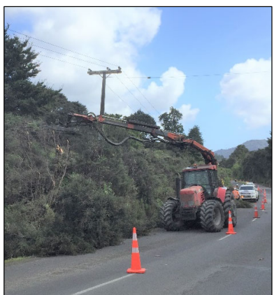
Shelter trimmer provides cost-effective tree work, removing the risk of people working on roadsides.
