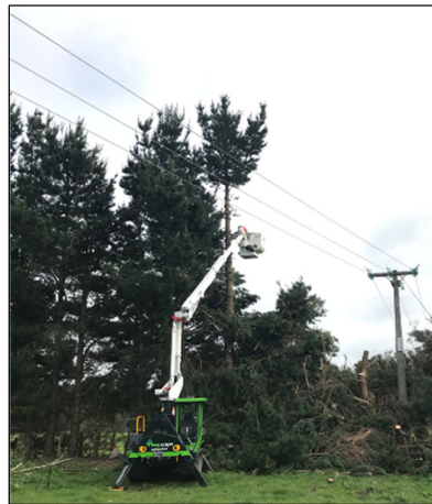
A tracked all-terrain elevated work platform allows easy access to trees as well as minimising the impact on surrounding land.
